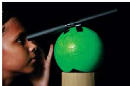
The diameter of the tube should be less than 2 cm. Fix the tube on a ball mount as in the figure.
