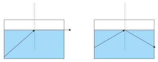
What happens as you increase the angle of incidence? Does the beam come out into air? Or does it reflect back into water as shown in this figure?
