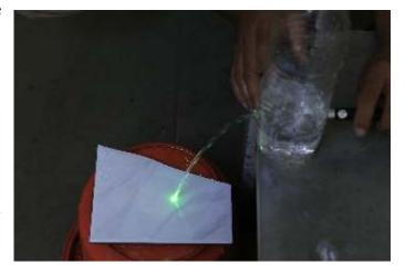
You will observe that the laser rays do not pass through the hole in straight direction, but they travel through the water jet, to fall in the bucket. The rays are bent along the path of jet.
